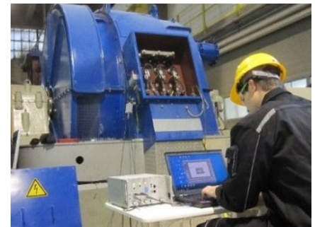
Fig. 9: Calibration of couplers for online PD measurements
