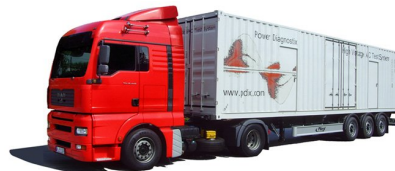
Fig. 1: 1.3 MW converter based test system
