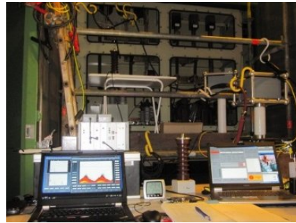
Fig. 7: On-site PD and TD test on a 150 MVA turbo generator
