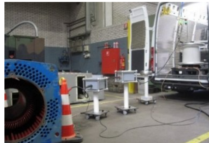
Fig. 8: Test setup on 250 kW asynchronous motor with the MV test van
