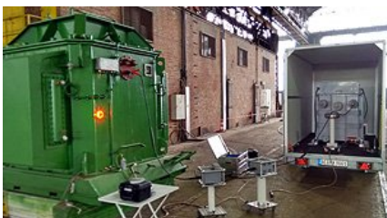
Fig. 6: On-site test on a 4500 MVA pump motor with the resonant test system
