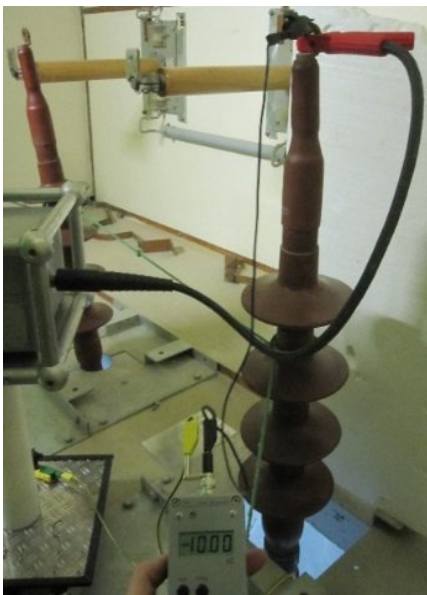
Fig. 11: PD calibration prior to an off-line PD test
