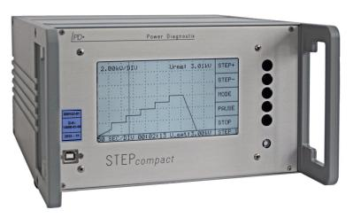
Increasing the high voltage stepwise is a task that is often required during type testing and production testing of high voltage equipment. The STEP*compact* is an instrument to automate such step tests. The unit combines the control function with the measurement capabilities of a high voltage meter.
