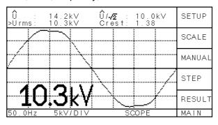
In the standard configuration, the STEPcompact comes with a self-contained relay box that is remotely controlled via a fiber optic cable. Alternatively, a direct connection to the HVcontrol, Power Diagnostix' standard control unit for high voltage test sets, can be provided. Using either the fiber optic transmission or the HVcontrol, the UP and DOWN relay contacts of the voltage regulator are actuated to adjust the high voltage according to the programmed test sequence.
