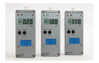
The appropriate choice of a calibration instrument depends on the range of typical charge values of the partial discharges being measured.
