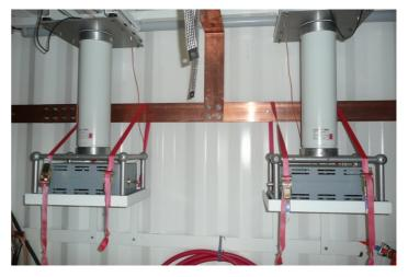
The voltage measurement signal can be taken from the capacitive divider on low voltage potential. This signal is directly connected via RG213 coaxial cable to the input of the Power Analyzer.
