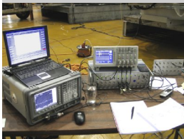
Advanced PD test system
