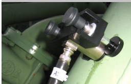
Acoustic sensor with magnetic holder
