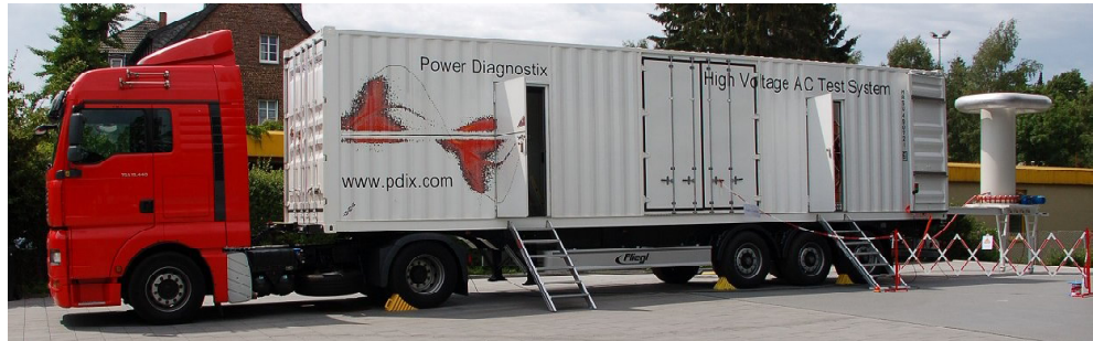
Test system with moved out reactor
