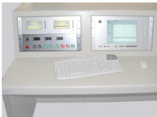
HVcontrol embedded in a control desk
